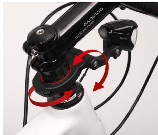
e. Bring angle of lightarm in position to get enough space for cables. Sometimes cables have to be placed in any other position.
