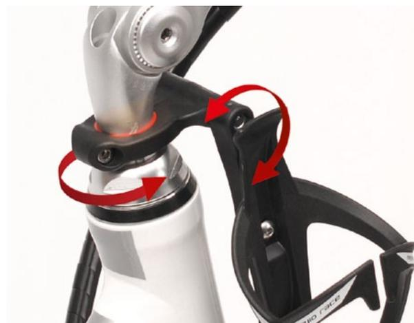
e. Bring angle in position to get enough space for cables and removal of bottle.
