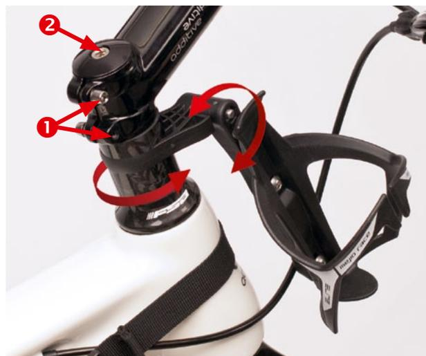
**b.** Untighten both screws (1) of stem. Screw (2) with cap has to be taken away as well as stem with bar. Spacer of your choice has to be replaced by Spacer One. Place Spacer One therefore in front direction and assemble stem and bar in reverse order. Now fix screw (2) only as hard as head set will turn easily. Then fix both screws (1) with torque 5Nm.
